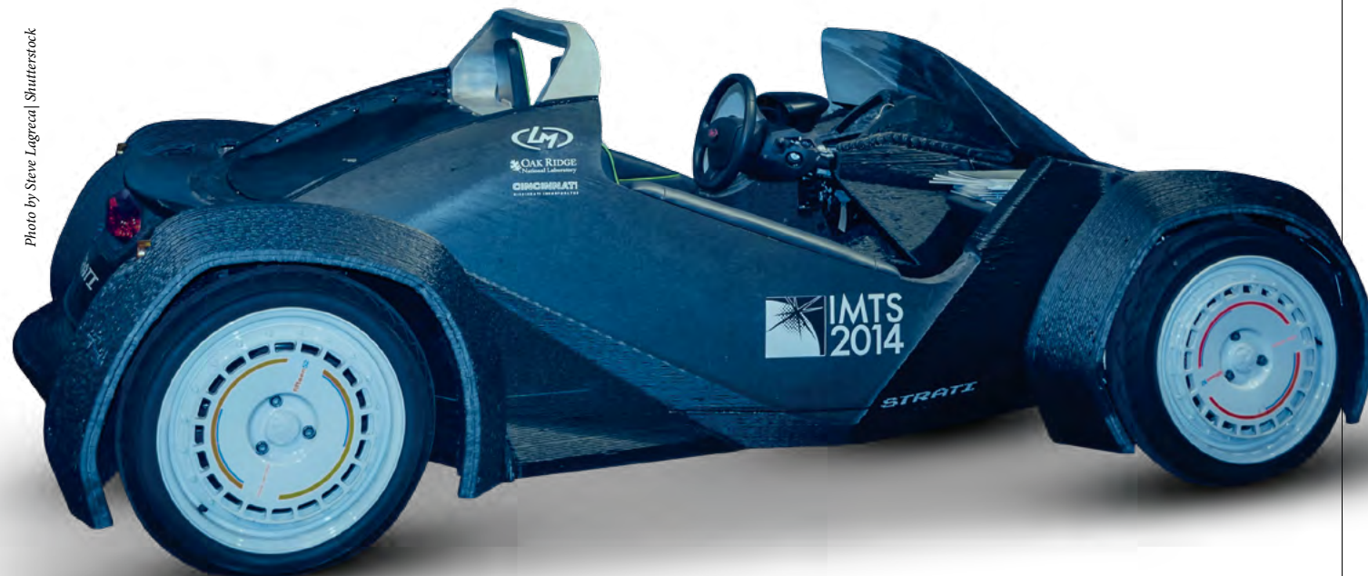
Local Motors Strati, a 3D-printed concept car, at The Gallery, an event sponsored by the North American International Auto Show (NAIAS) and the MGM Grand Detroit.
