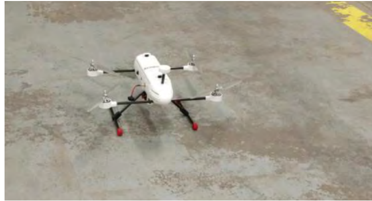
Fig 5.0 Flight testing the drone after assembly of parts including 3D printed parts
